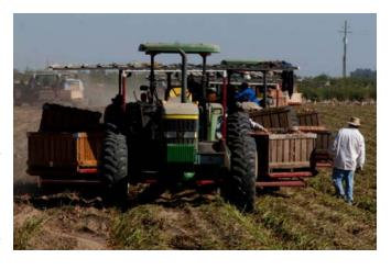
maximize the crop yields, the sweet potato harvester requires a team of workers to ride on them as they are drawn through the fields. The harvester consists of a tractor and a trailer. As the trailer is pulled along the field by the tractor, it digs the potatoes out of the ground and workers on the trailer separate the potatoes and put them into large bins. This part of the process works well and is an efficient use of man-power.
